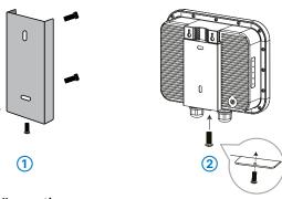
Use the mounting plate (1) as a drilling template to mark the
