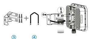
First screw the angle bracket (3) to the access point housing using the provided screws. Note the positioning of the washers and lock washers directly under the screw head. Then position the angle bracket with the screwed-on access point on the mast, guide the bracket 4 around the mast through the holes of the angle bracket and fasten it with the enclosed nuts after aligning the access point.
