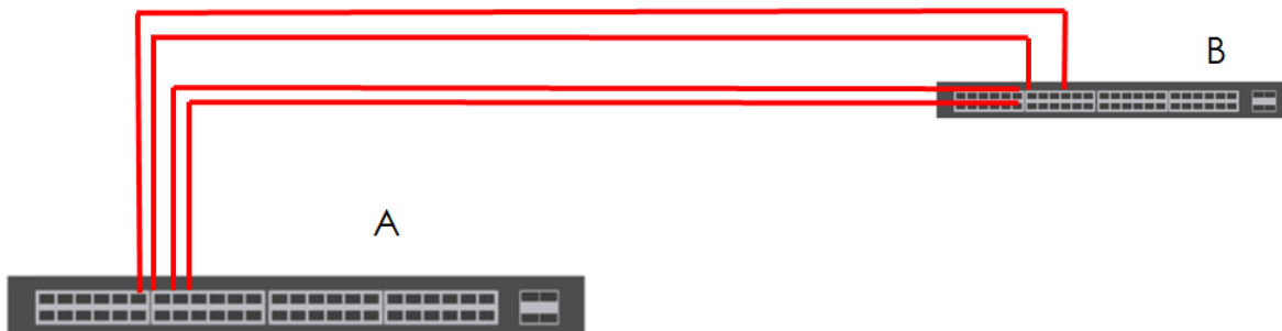
Figure 122 Trunking Example – Physical Connections
