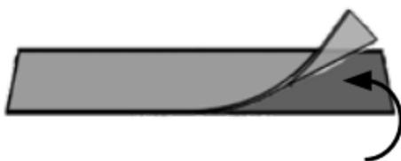
5. Place the thermal pad (side without foil downwards) directly onto the M.2 NVMe SSD and remove the second transparent protection foil now.
